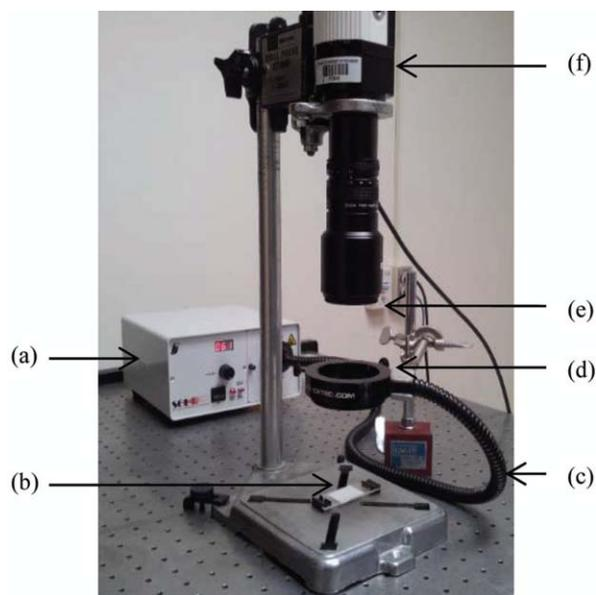
**FIGURE 1.** NIRF imaging system used for fluorescence imaging: (a) tungsten halogen light source (150 W), (b) Specimen, (c) fiber optics, (d) ring light source (785 nm), (e) band-pass filter (835 ± 37 nm), and (f) camera. [Color figure can be viewed in the online issue, which is available at [wileyonlinelibrary.com](http://wileyonlinelibrary.com).]
