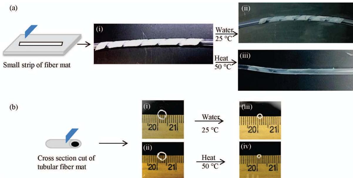
**FIGURE 6.** (a) A small strip was cut from the electrospun fiber mat and then wrapped around a pediatric catheter tube (i). The strip was shrunk on to the tube by applying (ii) 25°C water or (iii) 50°C heat. (b) Small rings were cut from a halo tube of electrospun fiber mat [(i) and (ii)] and recovered by applying (iii) 25°C water and (iv) 50°C heat. [Color figure can be viewed in the online issue, which is available at [wileyonlinelibrary.com](http://wileyonlinelibrary.com).]
