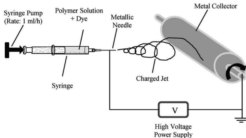
**SCHEME 1.** Schematic of electrospinning device.
