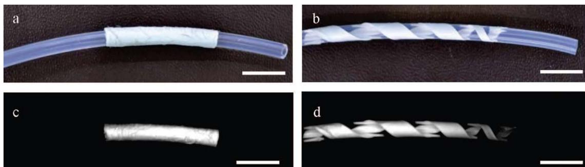
**FIGURE 7.** (a) and (b) are photographs of electrospun tube and small strip cut from electrospun fiber mat of PVAc/ICG with the ICG concentration of 0.0125 mg/mL wrapped around a pediatric catheter tube. (c) and (d) are the NIRF images of same devices taken with the gain of 1.0 and exposure time of 140 ms. The scale bar represents 10 mm. [Color figure can be viewed in the online issue, which is available at [wileyonlinelibrary.com](http://wileyonlinelibrary.com).]
