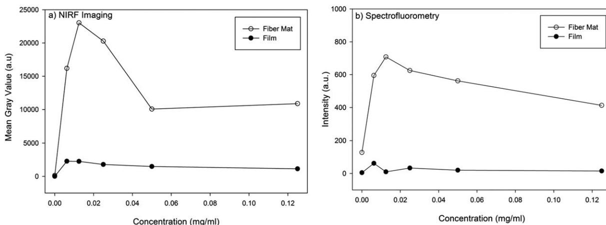
**FIGURE 5.** Graph of comparison of PVAc fiber mat and PVAc film with different ICG concentration by using (a) NIRF imaging and (b) Spectrofluorometry. The mean gray values were computed by using ImageJ program. PVAc fiber mat showed higher intensity and mean gray values compared to the PVAc film. The highest intensity by spectrofluorometry and the highest mean gray value by NIRF imaging were observed for samples with 0.0125 mg/mL ICG concentration.
