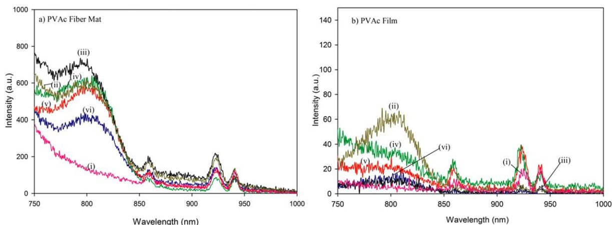
**FIGURE 4.** Spectrofluorometry of (a) PVAc fiber mat with different ICG concentration, and (b) PVAc films with ICG concentration of (i) 0 mg/mL, (ii) 0.00625, (iii) 0.0125, (iv) 0.025, (v) 0.05, and (vi) 0.125. [Color figure can be viewed in the online issue, which is available at [wileyonlinelibrary.com](http://wileyonlinelibrary.com).]
