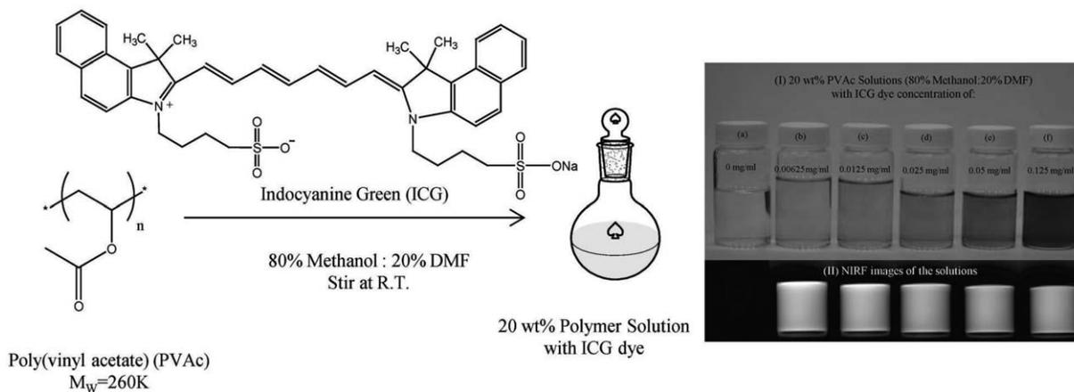
**SCHEME 2.** Procedure of incorporating ICG dye into the polymer solution. (I) The photograph of the solutions at ICG concentrations of (a) 0 mg/mL, (b) 0.00625 mg/mL, (c) 0.0125 mg/mL, (d) 0.025 mg/mL, (e) 0.05 mg/mL, and (f) 0.125 mg/mL. (II) The NIRF images of the same vials under the NIRF imaging system at the gain of 1 and exposure time of 150 ms.
