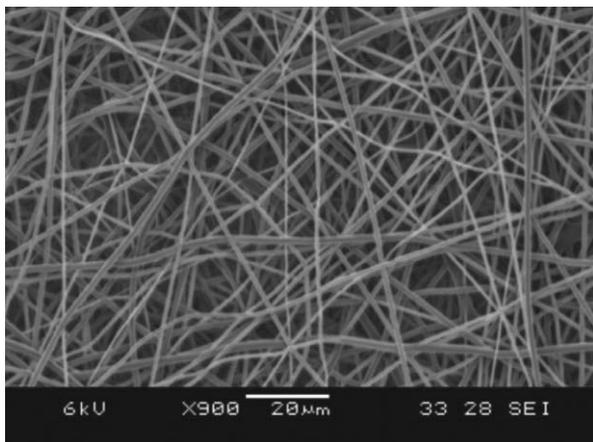
**FIGURE 2.** SEM image of electrospun PVA/ICG with the ICG concentration of 0.025 mg/mL with an average fiber diameter of  $0.86 \pm 0.22 \mu\text{m}$  ( $n=74$ ). ImageJ software was utilized to calculate the average fiber diameter.
