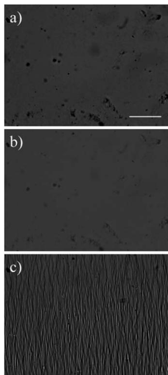
**Fig. 5** Optical micrographs of water triggered wrinkle formation with a 100 s gold coating and 12% prestrain. (a) In water at 30 °C for 5 h. (b) In water at 30 °C for 29 h. (c) In water at 30 °C for 5 h followed by 37 °C for an additional 24 h. The scale bar is 50  $\mu\text{m}$  and applies to all three images.
