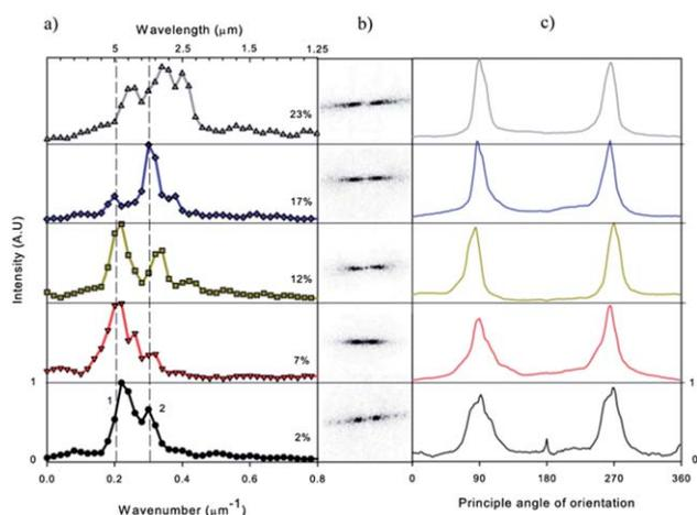
**Fig. 3** Characterization of wrinkles using 2D FFT. (a) Wavelength distributions of uniaxial wrinkles with a controlled thickness of gold and varying prestrain, (b) 2D FFT pattern of wrinkled surfaces, (c) relative degree of alignment characterization using 2D FFT pattern. "1" and "2" in the left frame indicate the first and second populations of uniaxial wrinkle wavelengths.
