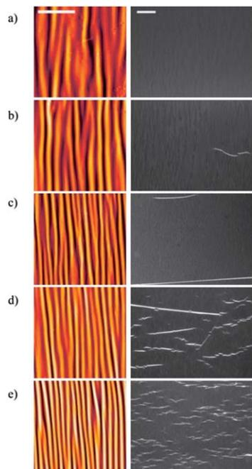
**Fig. 2** AFM wrinkle images (left) and OM crack images (right) with prestrain values of (a) 2%, (b) 7%, (c) 12%, (d) 17%, and (e) 23%. Heights in AFM images are given in color scale and range from  $z = 0$  nm black pixels to  $z = 700$  nm bright pixels. Scale bar is  $20 \mu\text{m}$  for AFM image (left) and  $200 \mu\text{m}$  for OM image (right).
