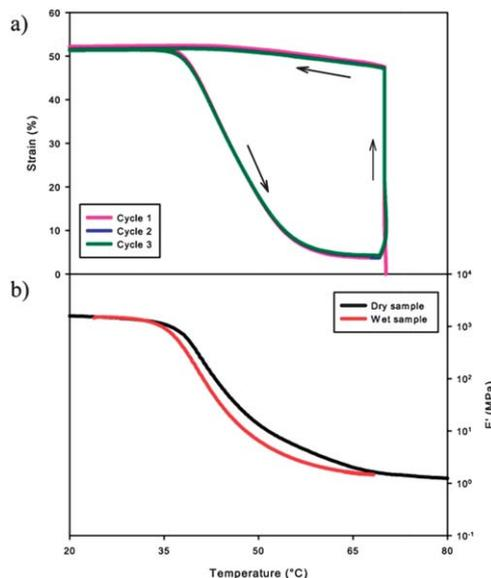
**Fig. 1** Thermomechanical properties of the *t*BA/BA substrate. (a) Shape memory cycle and (b) effect of temperature on tensile storage modulus for dry and hydrated samples.
