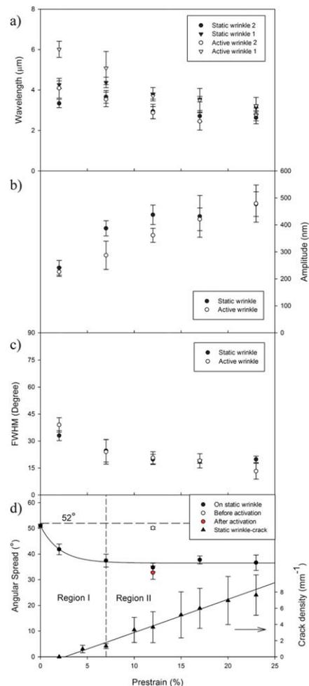
**Fig. 4** Characterization of static wrinkles and active wrinkles. (a) Wavelength change with respect to the prestrain, (b) amplitude dependence on wrinkle prestrain, (c) relative degree of alignment as a function of prestrain. (d) Cell orientation with respect to wrinkle prestrain. The controlled gold thickness in (a)–(d) is  $33 \text{ nm}$ . "1" and "2" in (a) indicate the first and second populations of uniaxial wrinkle wavelengths.
