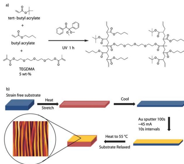
**Scheme 1** Process for fabricating the wrinkled material. (a) Chemical structure of synthesized substrate, (b) stretching, coating, and recovering the substrate to form wrinkles.
