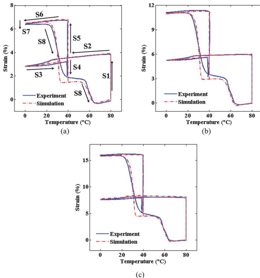
**Fig. 7** Model predictions for triple shape memory behaviors under three different nominal stress pairs. (a)  $P_1 = 0.1$  MPa,  $P_2 = 0.3$  MPa. (b)  $P_1 = 0.15$  MPa,  $P_2 = 0.45$  MPa. (c)  $P_1 = 0.2$  MPa,  $P_2 = 0.6$  MPa.
