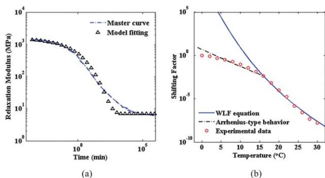
**Fig. 6** Model fitting for stress relaxation. (a) The stress relaxation master curve at 16 °C. (b) The shifting factors with temperature.
