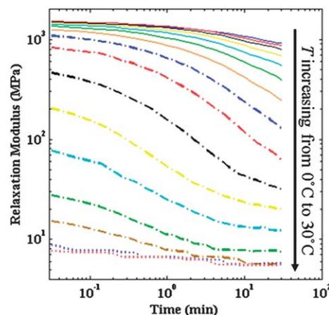
**Fig. 3** Tensile relaxation modulus for temperatures varying from 0 °C (indicate color or insert line) to 30 °C (indicate color or insert line) with 2 °C temperature intervals between experiments.
