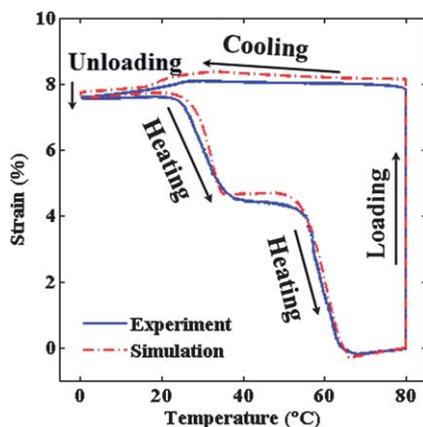
**Fig. 8** Comparisons between model prediction and experimental result for the one-step-fixing shape memory behavior.
