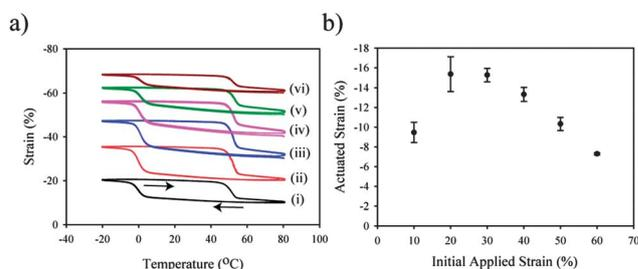
**Fig. 3** Two-way reversible actuation. (a) An 80PCL–20PEG SMP foam showed reversible two-way actuation of up to 15% when a constant load is applied during crystallization ((i) 10%, (ii) 20%, (iii) 30%, (iv) 40%, (v) 50%, and (vi) 60% initial applied strain); (b) a maximum actuation strain is observed with a prestrain of 30%, and the actuation strain decreases as the prestrain deviates from 30%.
