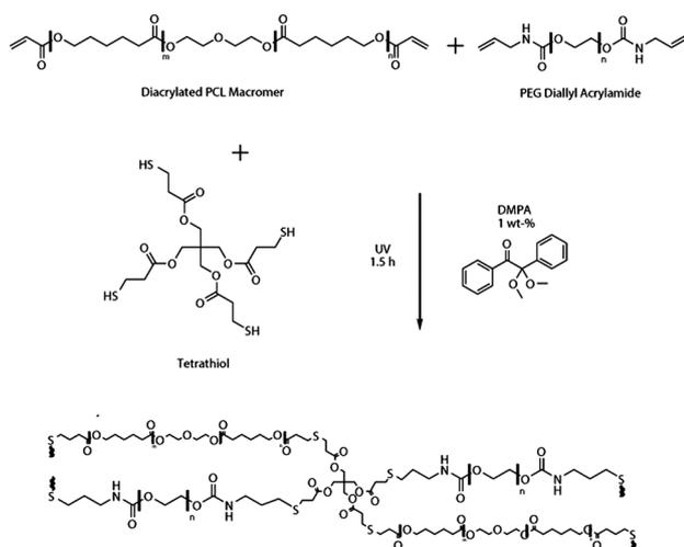
**Scheme 1** SMP network formation using photo-initiated addition reactions between oligomeric macromers and the shown tetrathiol.
