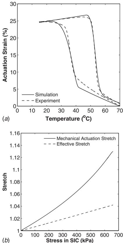
**Fig. 3 (a) Model fit to the experimental result for the case of imposed stress 700 kPa. (b) Comparisons between mechanical actuation stretch and effective stretch in SIC.**
