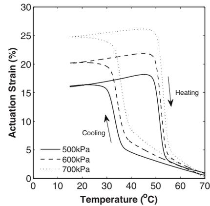
**Fig. 1 Two-way shape memory effects demonstrated by the PCO material under different stresses**
