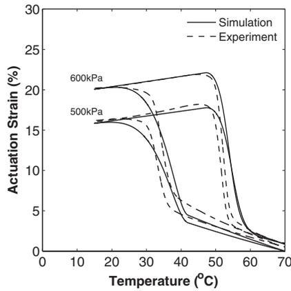
**Fig. 4 Comparisons between model predictions and experimental results for the case of 500 kPa and 600 kPa imposed stresses**
