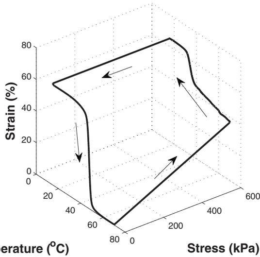
**Fig. 2 One-way SM effect demonstrated by PCO under 600 kPa stress**
