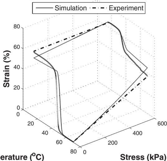
**Fig. 5 Comparison between the model simulation and the experiment for the one-way SM effect under 600 kPa stress**
