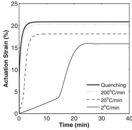
**Fig. 7 Effects of temperature rates on the actuation strain for the case of cooling followed by holding the sample**
