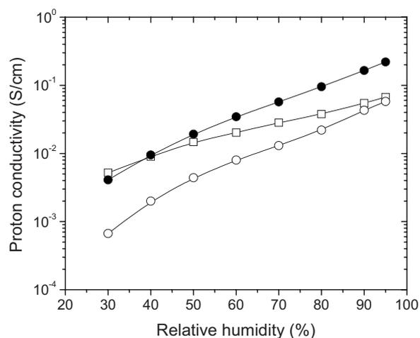
**Figure 6.** Proton conductivity as a function of RH at 30 $^{\circ}$ C for nanofiber network composite membranes. (●) sPAES/sPOSS (60/40 w/w), (○) 2.1 mmol/g sPAES (without sPOSS), and (□) Nafion 212. The fiber volume fraction of the nanofiber network composite membranes was 0.70 and 0.75 for sPAES/sPOSS (60/40 w/w) and sPAES (no sPOSS), respectively.
