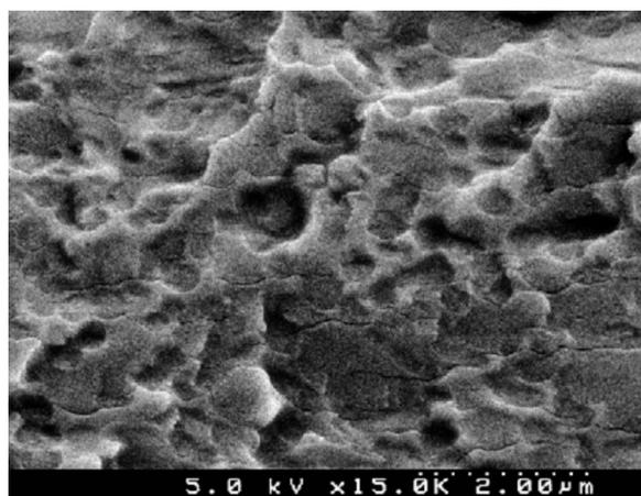
**Figure 5.** SEM of an embedded nanofiber network composite membrane cross section at a magnification of 15,000 $\times$ . Nanofibers were composed of 2.1 mmol/g sPAES with 40 wt % sPOSS. The inert matrix polymer was NOA 63.
