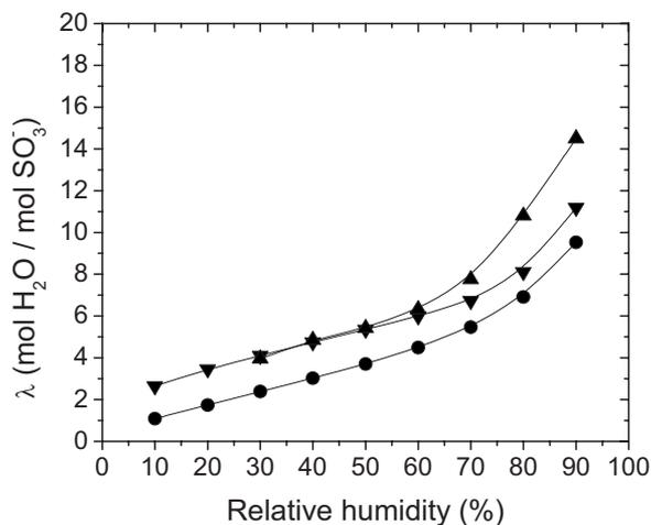
**Figure 9.** Hydration number ( $\lambda$ ) as a function of RH at 30°C for nanofiber composite membranes. (▲) sPAES/sPOSS (60/40 w/w), (▼) 2.1 mmol/g IEC sPAES (no sPOSS), and (●) Nafion 212. Fiber volume fraction of the nanofiber network composite membranes was 0.70 and 0.75 for sPAES/sPOSS (60/40 w/w) and sPAES, respectively.
