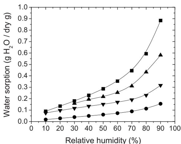
**Figure 8.** Equilibrium water-vapor sorption as a function of RH at 30°C (■) pure sPOSS, (▲) sPAES/sPOSS (60/40 w/w) nanofiber network membrane, (▼) 2.1 mmol/g IEC sPAES (no sPOSS) nanofiber network membrane, and (●) Nafion 212. Fiber volume fraction of the nanofiber network composite membranes was 0.70 and 0.75 for sPAES/sPOSS (60/40 w/w) and sPAES (no sPOSS), respectively.
