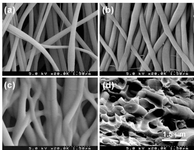
**Figure 3.** SEMs (20,000 $\times$  magnification) of nanofiber structures obtained after successive membrane fabrication steps: (a) Surface of the as-spun mat, (b) surface of mat after compaction, (c) surface after mat compaction and fiber welding, and (d) cross section of the final membrane after embedding with NOA 63 polymer. The nanofibers were composed of 2.1 mmol/g IEC sPAES.
