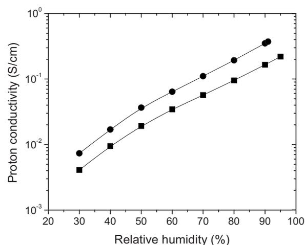
**Figure 7.** Proton conductivity dependence on RH for a nanofiber network composite membrane from sPAES (2.1 mmol/g IEC)/sPOSS (60/40 w/w) with a fiber volume fraction of 0.70. (■) 30 and (●) 80 $^{\circ}$ C.
