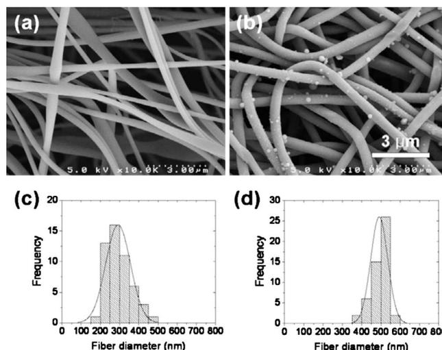
**Figure 4.** SEMs of (a) 2.1 mmol/g IEC sPAES, (b) 2.1 mmol/g IEC sPAES/sPOSS (60/40 w/w) nanofiber mats electrospun from 2-butoxyethanol at a magnification of 10,000 $\times$ , (c) fiber diameter distribution histogram of 2.1 mmol/g sPAES nanofiber mat, and (d) fiber diameter distribution histogram of sPAES/sPOSS mat.
