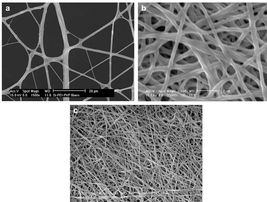
Fig. 2. SEM images of the silicified electrospun fibers of PEI:PVP (50:50) corresponding to the electrospun fibers of (a) Fig. 1a and (b, c) Fig. 1b.
