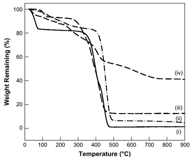
**Fig. 5.** TGA analysis of the silicified and non-silicified electrospun fibers of 50:50 blends of linear PEI and PVP (i) PEI:PVP fibers at ca. 40% humidity, (ii) silicified electrospun PVP fibers (control), (iii) silicified PEI:PVP fibers after exposure at ca. 40% humidity and (iv) silicified PEI:PVP fibers after exposure at ca. 80% humidity.
