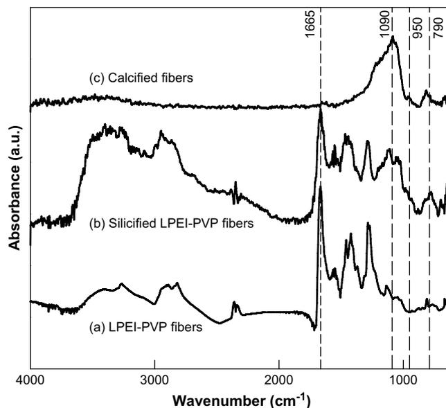
Fig. 7. FTIR of the electrospun PEI-PVP fibers (a) before silicification, (b) after silicification and (c) after calcination at  $600\text{ °C}$  for 1 h.
