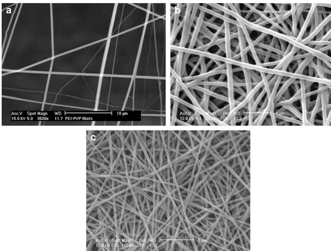
Fig. 1. SEM images of the fibers of the 50:50 blends of linear PEI and PVP in ethanol electrospun at concentration of (a) 5 wt% and (b, c) 10 wt%.
