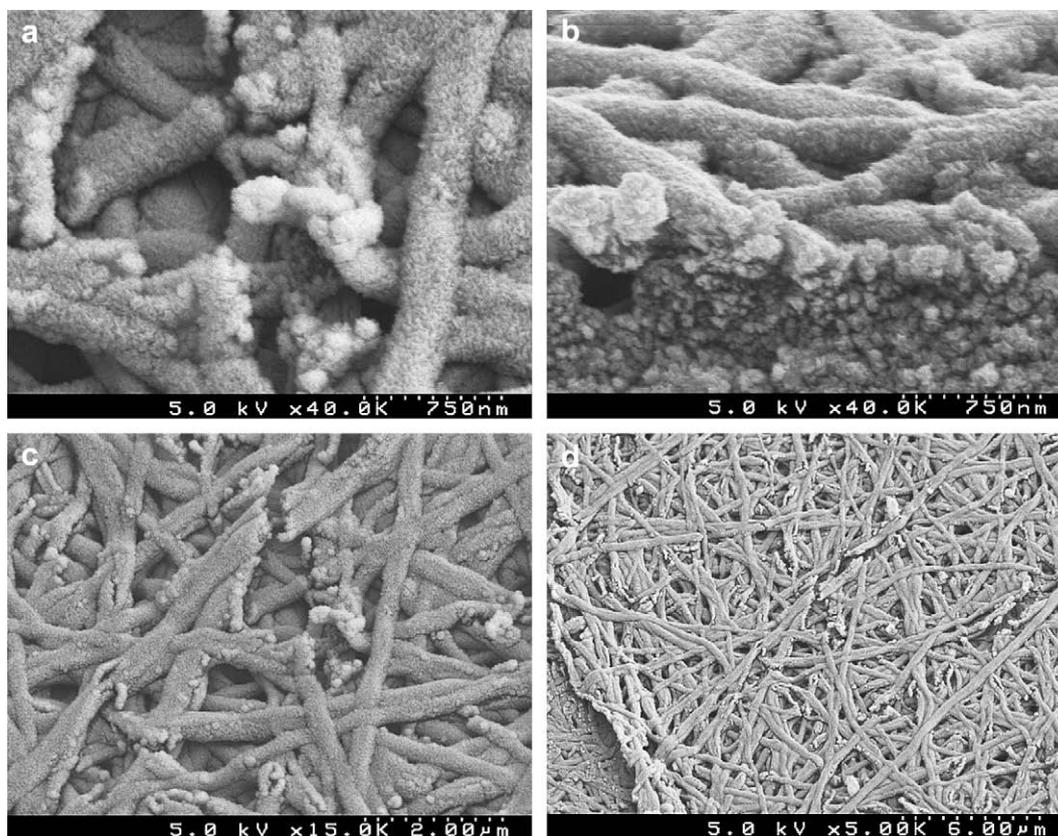
Fig. 6. High resolution SEM images of the silicified fibers after calcination at 600 °C for 1 h (a, c, d) top view and (b) cross-sectional view.
