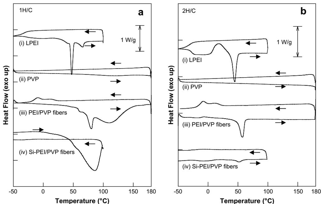
**Fig. 4.** DSC curve of the (a) first heating/cooling cycle and (b) second heating/cooling cycle of: (i) LPEI, (ii) PVP and (iii) LPEI/PVP e-spun fibers and (iv) Silicified LPEI/PVP e-spun fibers after TMOS immersion for 10 min. The heating and cooling is at rate of 10 °C/min.
