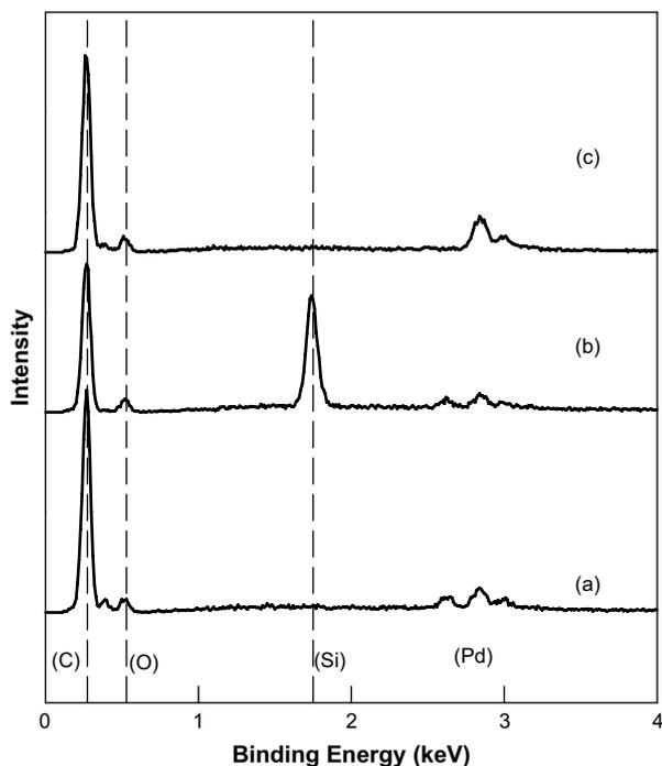
Fig. 3. Energy Dispersive X-ray (EDX) spectra of (a) PEI/PVP (50/50 w/w) electrospun fibers, (b) after silicification by TMOS and (c) control sample of PVP fibers after TMOS exposure for 10 min. The vertical dotted line indicates the reference peak of the corresponding elements shown in bracket.
