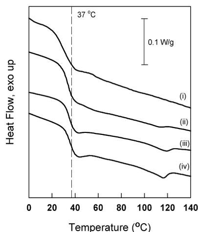
**Figure 3.** DSC second heating traces for (i) P(1k)LA-P0, (ii) P(1k)LA-P1, (iii) P(1k)LA-P2, and (iv) P(1k)LA-P3.
