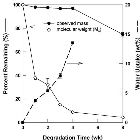
**Figure 7.** Degradation profile for P(1k)LA-P3, including percent observed mass remaining (●), percent number-average molecular weight ( $M_n$ ) remaining (◇), and weight percent water uptake (■).
