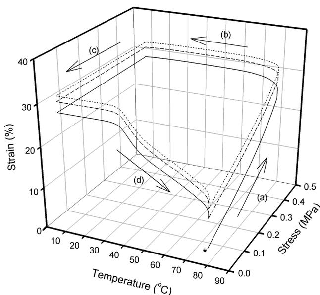
**Figure 6.** One-way shape memory cycles for P(1k)LA-P3. Three cycles are shown: (—) first cycle, (---) second cycle, and (- · -) third cycle. The asterisk marks the beginning of the cycle and the arrows denote the various stages, specifically (a) deformation, (b) cooling/fixing, (c) unloading, and (d) recovery.
