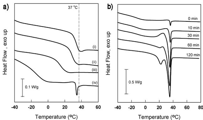
**Figure 1.** DSC second heating traces for (a) **P(x)LA** polyols initiated by PEG with molecular weights of (i) 600 g/mol, (ii) 1 kg/mol, (iii) 2 kg/mol, (iv) 4 kg/mol; and (b) **P(4k)LA** with various annealing times at 10 °C showing the crystallization of the PEG block.
