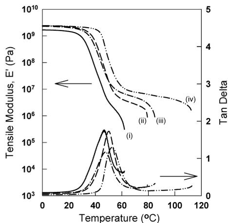
**Figure 5.** Storage tensile modulus measurements for TPUs with different POSS loadings: (i) P(1k)LA-P0, (ii) P(1k)LA-P1, (iii) P(1k)LA-P2, and (iv) P(1k)LA-P3.
