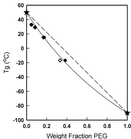
**Figure 2.** Change in  $T_g$  for **P(x)LA** polyols with different molecular weight PEG initiator as calculated from an ideal 12 kDa composition ( $\diamond$ ) and using molecular weight determined by NMR ( $\bullet$ ). PEG 0% (all lactide)<sup>63</sup> and PEG 100% ( $M_w = 10$  kg/mol)<sup>64</sup>  $T_g$  values are taken from the indicated references. The dashed line connects the two extremes and represents the Fox equation. The curved solid line is a fit to the Gordon–Taylor equation.
