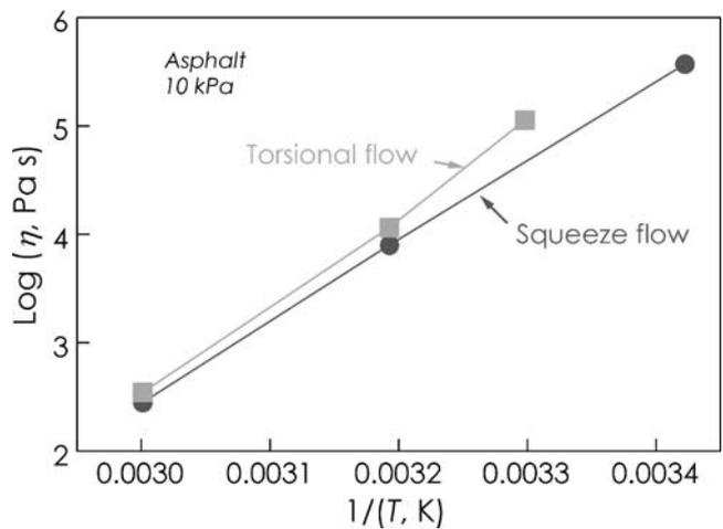
**Fig. 9** Viscosity changes with temperature for asphalt as measured by the two techniques at a stress of 10 kPa. The Cox–Merz relationship is assumed for conversion of the complex viscosity magnitude to steady shear viscosity
