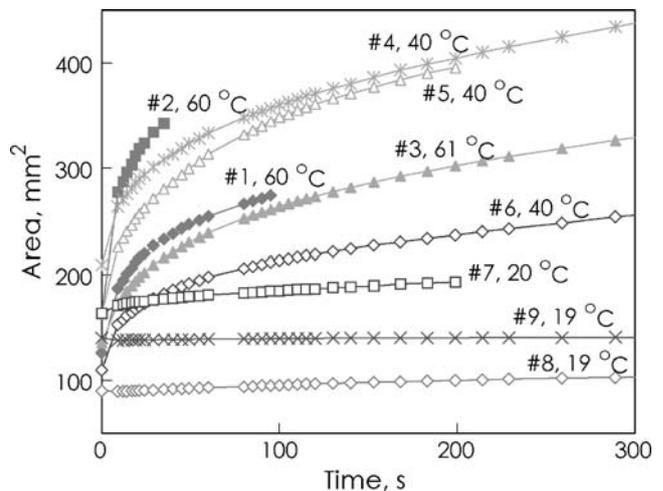
**Fig. 5** Sample area change as a function of time during a squeeze-flow run
