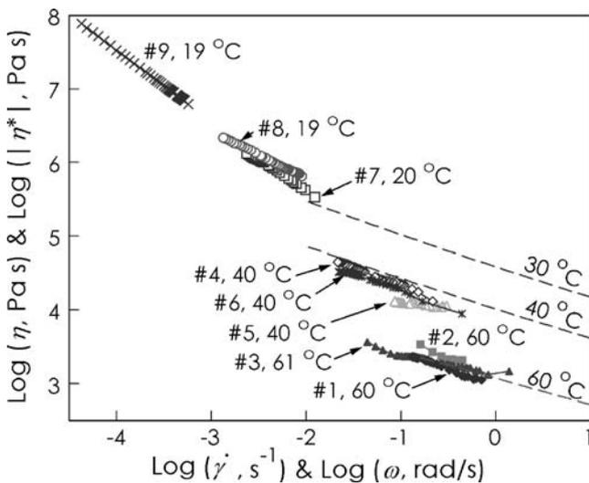
**Fig. 8** Comparison of viscosity results obtained from combinatorial rheometer with the magnitude of the complex viscosity (dotted lines) obtained using parallel-plate fixtures in an Advanced Rheometric Expansion System (ARES) rheometer
