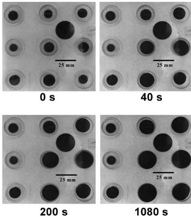
**Fig. 4** Images taken during a combinatorial squeeze flow run at the times indicated. The partial vacuum is 76 mmHg, while the temperatures of the vertical rows are 20, 40, and 61 °C left to right. The black circle in the upper right quadrant is a size scale reference
