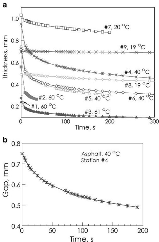
**Fig. 6** **a** Sample thickness during a single combinatorial squeeze-flow run derived from area; and **b** example fit of the integral form of the Scott equation to observations for Station #4. The first point has been eliminated, and the time scale shifted. Power-law constants:  $m=7070\pm 400$  and  $n=0.572\pm 0.024$ . Initial gap:  $0.735\pm 0.008$  mm
