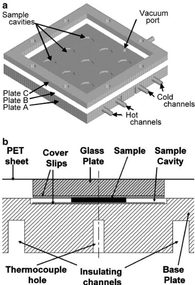
**Fig. 2** Combinatorial instrumental setup. **a** Pictorial view and **b** cross-section of one cell
