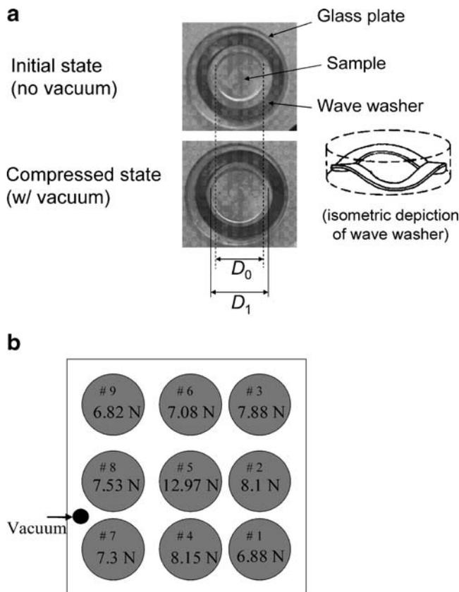
**Fig. 3** **a** Images of a squeeze cell before and after application of partial vacuum. The clear sample of silicone has been squeezed in the bottom photo to a larger diameter  $D_1$  than the starting size  $D_0$  in the top photo. The *dark ring* is the wave washer, which is compressed in the bottom photo by a ratio  $(D_1/D_0)^2$ . The *inset* is a sketch of a wave washer. **b** Sample positions and the average force calculated from the deflection of wave washers
