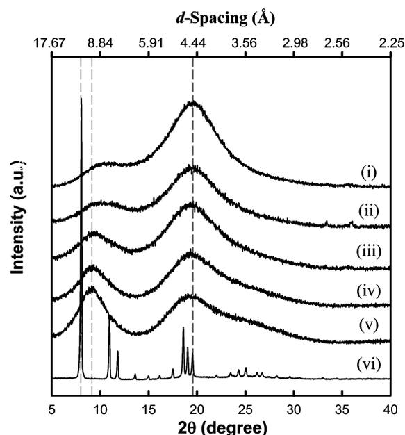
**Figure 2.** WAXS patterns of as-cast films of <sup>i</sup>BuPOSS–PS copolymers with varying weight percentage of <sup>i</sup>BuPOSS: (i) 0, (ii) 6, (iii) 15, (iv) 30, (v) 50 wt % <sup>i</sup>BuPOSS, and (vi) styryl <sup>i</sup>BuPOSS macromer.
