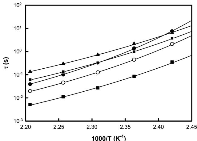
**Figure 13.** Temperature dependence of terminal zone relaxation time ( $\tau$ ) for as-cast films of  $i$ BuPOSS-PS copolymers as a function of POSS weight fraction: (●) 0, (○) 6, (■) 15, (□) 30, and (▲) 50 wt %  $i$ BuPOSS. The solid lines represent the best-fit VFTH curves for the copolymers and PS homopolymer.
