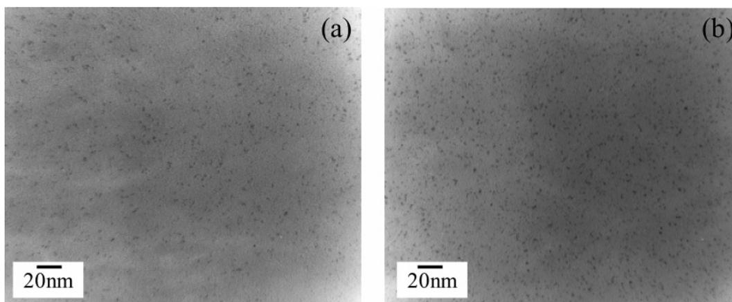
**Figure 3.** Transmission electron microscopy (TEM) images of as-cast films of <sup>t</sup>BuPOSS–PS copolymers: (a) 6, (b) 30 wt % <sup>t</sup>BuPOSS. The samples were stained by RuO<sub>4</sub> vapor at ambient condition.
