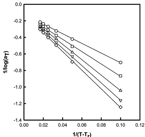
**Figure 7.** WLF function plot of shift factor for as-cast films of <sup>i</sup>BuPOSS-PS copolymers with varying weight percentage of <sup>i</sup>BuPOSS: (○) 0, (□) 6, (△) 15, (▽) 30, and (◇) 50 wt % POSS. The reference temperature is 120 °C.
