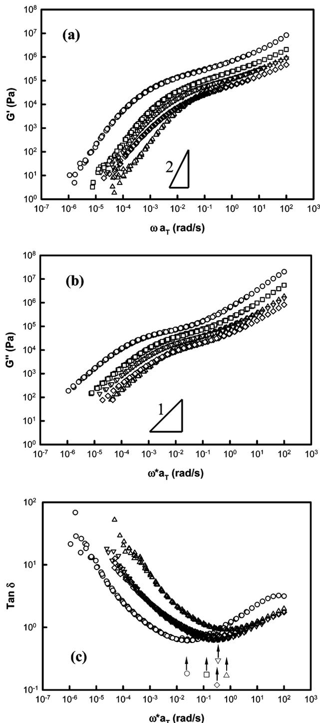
**Figure 6.** Master curve of as-cast films of <sup>i</sup>BuPOSS-PS copolymers with varying weight percentage of <sup>i</sup>BuPOSS: (○) 0, (□) 6, (△) 15, (▽) 30, and (◇) 50 wt % <sup>i</sup>BuPOSS with  $T_r = 120$  °C: (a)  $G'$ , (b)  $G''$ , and (c)  $\tan \delta$ . The arrows in (c) indicate the minimum values of  $\tan \delta$  for each sample.
