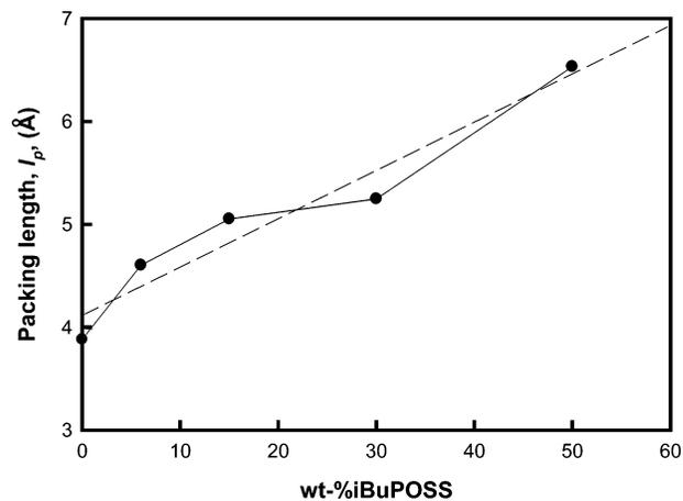
**Figure 10.** Plot of packing length ( $l_p$ ) of as-cast films of <sup>i</sup>BuPOSS–PS copolymers with varying weight percentage of <sup>i</sup>BuPOSS as a function of <sup>i</sup>BuPOSS weight fraction. The packing length is calculated using eq 13.
