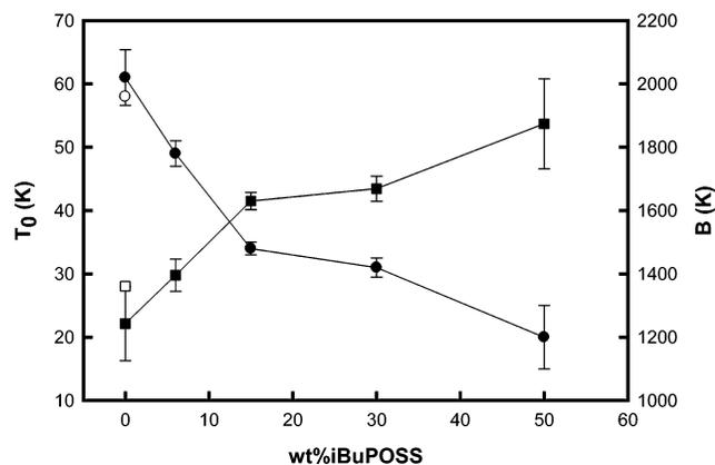
**Figure 14.** Plot of Vogel temperature ( $T_0$ , ●) and apparent activation energy ( $B$ , ■) of  $i$ BuPOSS–PS copolymers as a function of  $i$ BuPOSS content, which are extracted from the best-fit curves shown in Figure 14. The symbols of open circle (○) and open square (□) are the values of  $T_0$  and  $B$  for PS from ref 51.
