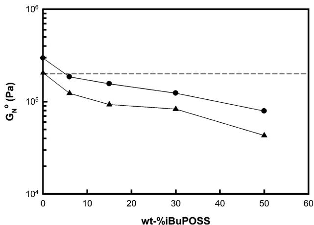
**Figure 9.** Rubbery plateau modulus ( $G_N^o$ ) as a function of <sup>i</sup>BuPOSS weight fraction: (●) evaluated using eq 9 and (▲) determined from  $G'$  at minimum  $\tan \delta$ . The dashed reference line is the plateau modulus of PS reported in ref 36.
