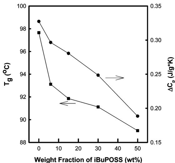
**Figure 5.** Variation of glass-transition temperature (■,  $T_g$ ) and heat capacity step change (●,  $\Delta C_p$ ) at  $T_g$  as functions of <sup>i</sup>BuPOSS content.  $T_g$  is determined from the midpoint of enthalpy change in the DSC trace curves shown in Figure 4.
