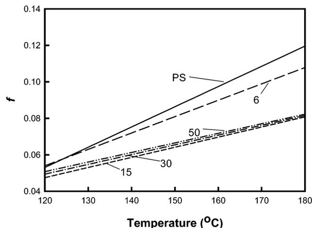
**Figure 8.** Temperature dependence of fractional free volume ( $f$ ) as-cast films of <sup>i</sup>BuPOSS-PS copolymers with varying weight percentage of <sup>i</sup>BuPOSS: (—) 0, (---) 6, (-·-·-) 15, (-·-·-·-) 30, and (····) 50 wt % POSS.
