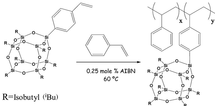
**Figure 1.** Synthetic scheme for the preparation of random copolymers yielded from styrene– and styryl–isobutylPOSS (<sup>i</sup>BuPOSS) through radical copolymerization initialized by AIBN at 60 °C.
