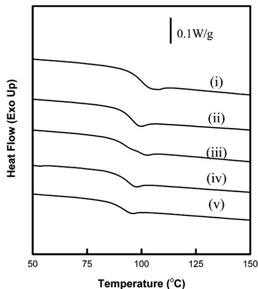
**Figure 4.** Differential scanning calorimetry (DSC) analysis of as-cast <sup>t</sup>BuPOSS–PS copolymers films with varying weight percentage of <sup>t</sup>BuPOSS: (i) 0, (ii) 6, (iii) 15, (iv) 30, and (v) 50 wt % <sup>t</sup>BuPOSS. The heating rate was 10 °C/min, and the second heating traces are shown.
