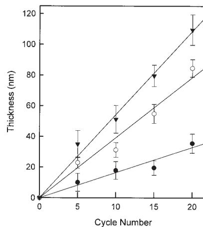
**Figure 8.** Thickness from AFM versus cycle number for spin assembly of PSS/PAH films using different salt concentrations: No salt (●);  $0.01 M$  (○); and  $2.0 M$  (▼). The solid lines represent linear regressions.
