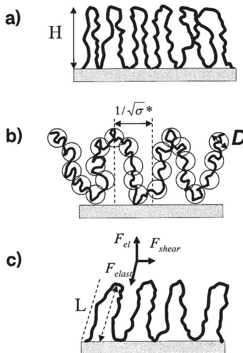
**Figure 10.** Schematic representation of the adsorbed layer (a) without shear; (b) without shear and with indication of Pincus blobs; and (c) under applied shear.
