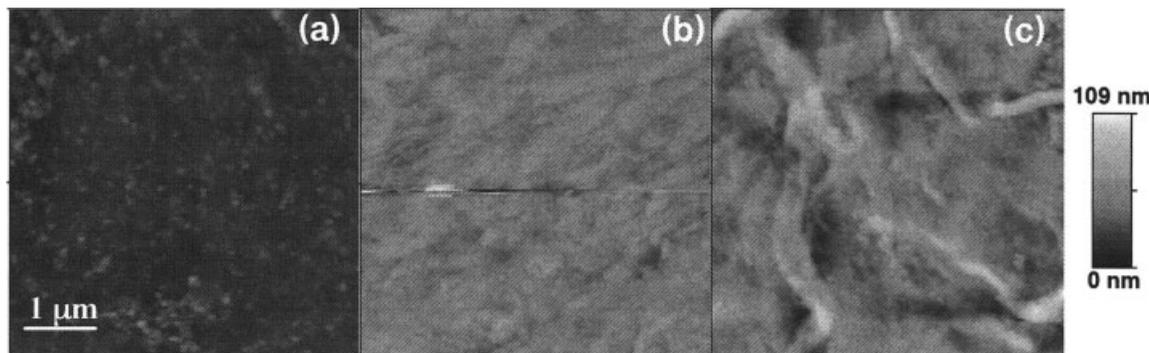
**Figure 5.** AFM images of the morphology of 20 bilayer films of PSS/PAH ( $10^{-2}$  M, pH = 3.5) deposited by the spin assembly process from: (a) 0 M, (b) 0.5 M, and (c) 2 M NaCl solutions.
