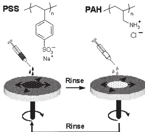
**Scheme 1.** Spin self-assembly process (3000 rpm during 8 s with a rinse step in between) and the chemical structures of the polyanion and polycation, poly(styrene sodium sulfonate) (PSS) and poly(allylamine hydrochloride) (PAH), respectively.
