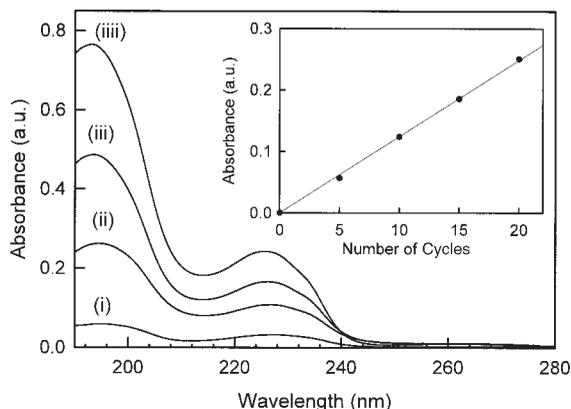
**Figure 1.** Plot of the absorbance versus wavelength of PSS/PAH ( $10^{-2} M$ , pH = 3.5) for a salt concentration of 0.1 M preparing by spin assembly at different number of bilayers: (i) 5 (i); (ii) 10; (iii) 15; and (iv) 20. Spin conditions: 3000 rpm, 8 s. Inset is peak absorbance (225 nm) versus cycle number of PSS/PAH ( $10^{-2} M$ , pH = 3.5) for 0.1 M NaCl concentration in both solutions. The solid line is a linear regression of the data.
