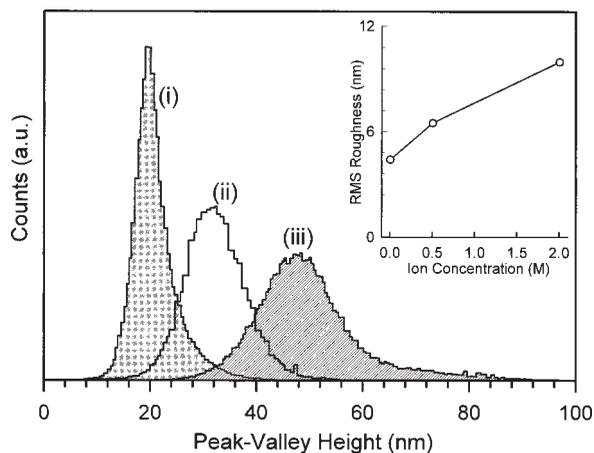
**Figure 6.** Peak-valley height distributions for different NaCl concentrations: (i) 0 M; (ii) 0.5 M; and (iii) 2 M. Inset is RMS roughness versus salt concentration.
