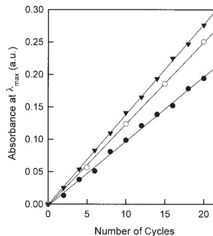
**Figure 2.** Plot of the absorbance at 225 nm versus the number of deposition cycles of PSS/PAH ( $C = 10^{-2} M$ , pH = 3.5) for varying NaCl concentration: No salt ( $\bullet$ ); 0.1 M ( $\circ$ ); 2.0 M ( $\blacktriangledown$ ) in both polyelectrolyte solutions preparing by spin assembly (3000 rpm, 8 s). Solid lines represent linear regressions.
