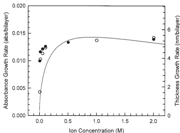
**Figure 9.** Thickness (○) and absorbance at 225 nm (●) at (PSS/PAH)<sub>20</sub> versus salt concentration, films prepared with Polyelectrolyte Spin Assembly method (3000 rpm, 8 s,  $C = 10^{-2}$  M, pH = 3.5).
