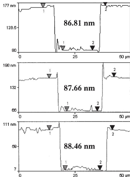
**Figure 7.** Thickness measurements are obtained by scratching with a razor blade to remove all the polyelectrolytes multilayer film. Dark side in the AFM image represents the scratch. Thickness measurements are made at several points (15 points). For instance, AFM from a 20 bilayers film of PSS/PAH ( $C = 10^{-2} M$ ,  $\text{pH} = 3.5$ ) with a  $0.05 M$  salt concentration: Thickness  $0.8831 \pm 1.98 \text{ nm}$ .
