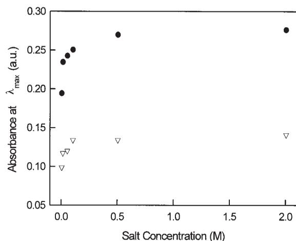
**Figure 4.** Absorbance values at 225 nm for 10 ( $\nabla$ ) and 20 ( $\bullet$ ) spin assembly cycles of PSS/PAH ( $10^{-2} M$ ,  $\text{pH} = 3.5$ ) versus NaCl concentration. The reported absorbance was measured at the rotation axis center.
