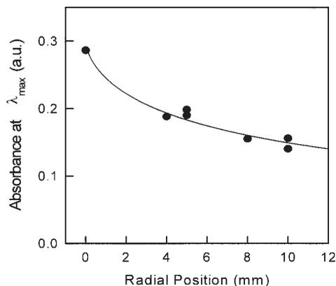
**Figure 3.** Radial dependence of the absorbance at 225 nm after 20 cycles of deposition of PSS/PAH ( $C = 10^{-2} M$ ,  $\text{pH} = 3.5$ ) and NaCl concentration of 0.5 M. The solid line represents the best fit of eq 5 to the experimental data.
