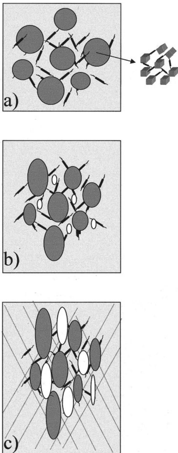
**Figure 9.** Schematic deformation process: (a) undeformed stage, (b) earlier stage of plastic deformation under a tensile load, and (c) advanced stage of plastic deformation. In parts b and c, the light regions represent nucleated voids.
