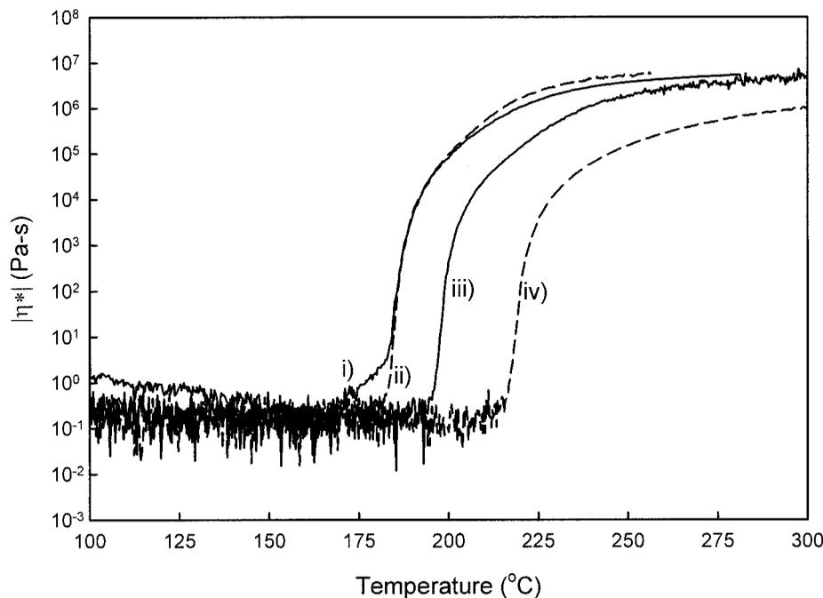
**Figure 2.** Temperature dependence of the complex viscosity ( $|\eta^*|$ ) for OG-POSS/DDS epoxies undergoing cure with (i) 100, (ii) 75, (iii) 50, and (iv) 25% of the stoichiometric ratio of DDS. The heating rate was 2 °C/min, and the oscillation frequency was 10 rad/s.
