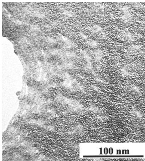
**Figure 8.** Representative deformation structure taken from an OG-POSS epoxy with 100% of the stoichiometric ratio of DDS. The image contrast was enhanced with Adobe Photoshop to highlight the apparent aggregation structures.
