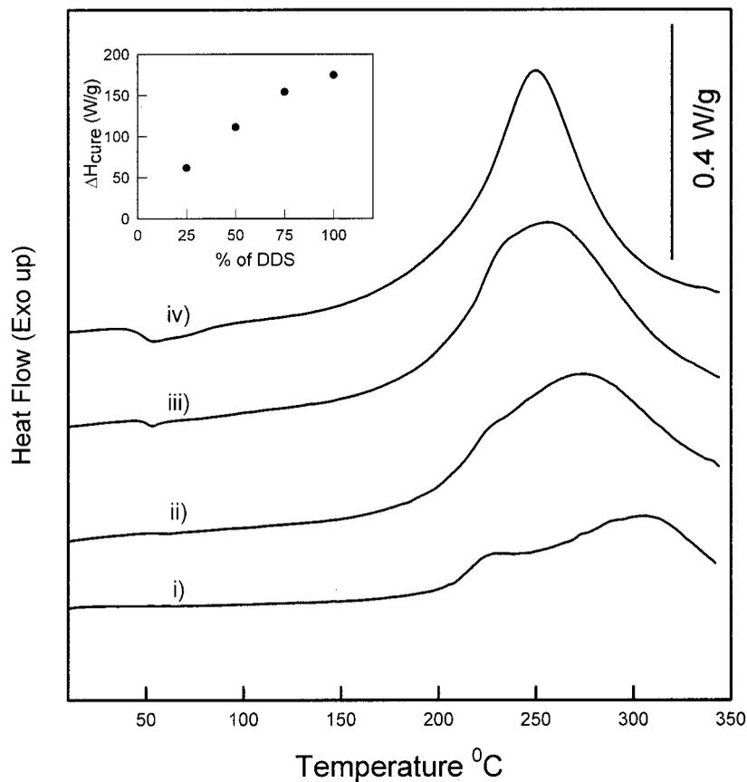
**Figure 1.** DSC for OG-POSS/DDS epoxies with (i) 25, (ii) 50, (iii) 75, and (iv) 100% of the stoichiometric ratio of DDS. The inset graph shows a plot of  $\Delta H_{\text{cure}}$  versus the stoichiometric ratio of DDS. A heating rate of 10 °C/min was used with a blanket of gaseous nitrogen.
