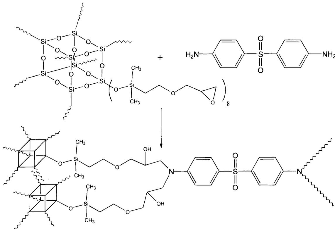
**Scheme 2.** Postulated reaction of OG-POSS with the four functional groups of DDS (two primary amines and two secondary amines). Such epoxy-amine reactions are commonly autocatalytic in nature because of an accelerating effect of the hydroxyls formed during epoxide ring opening.
