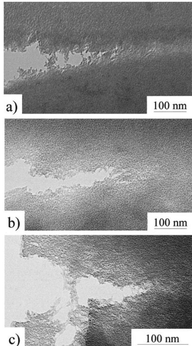
**Figure 7.** TEM micrographs revealing deformation structures of OG-POSS/DDS epoxies with (a) 50, (b) 75, and (c) 100% of the stoichiometric DDS ratio. The samples were stained with  $\text{RuO}_4$  and randomly microtomed; this caused damage that could be visualized.
