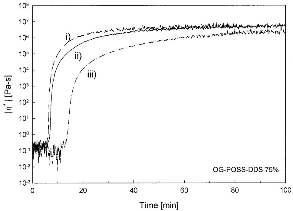
**Figure 3.** Evolution of the complex viscosity ( $|\eta^*|$ ) measured at a frequency of 10 rad/s during the isothermal curing of OG-POSS/DDS epoxies with different amounts of DDS at (i) 220, (ii) 200, and (iii) 180 °C. The stoichiometric percentage of DDS used is indicated in each plot.
