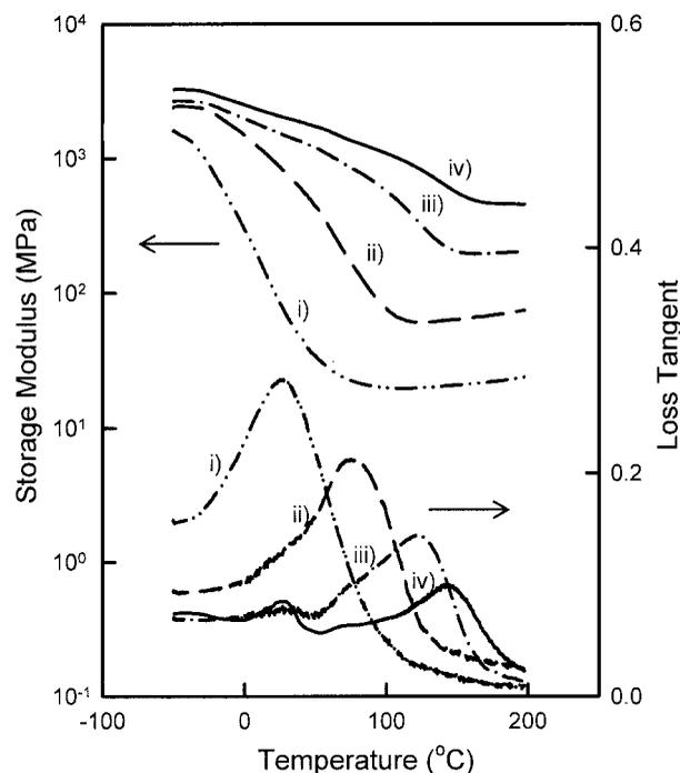
**Figure 4.** Tensile storage modulus and loss tangent of OG-POSS/DDS epoxies with (i) 25, (ii) 50, (iii) 75, and (iv) 100% of the stoichiometric ratio of DDS. A three-point-bending geometry was used with an oscillation frequency of 1 Hz and a heating rate of 4 °C/min.
