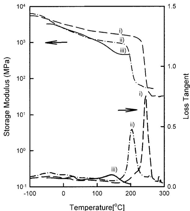
**Figure 5.** Tensile storage modulus and loss tangent for (i) DGEBA/DDS, (ii) OG-DGEBA (50:50 w/w)/DDS, and (iii) OG-POSS/DDS. A stoichiometric ratio of epoxide to amine was used. The conditions are described in Figure 4.
