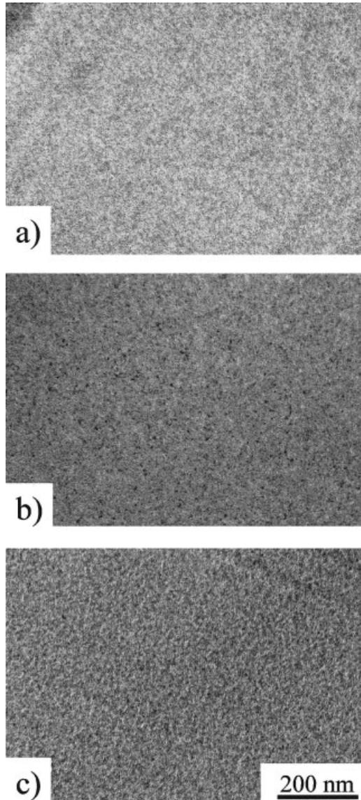
**Figure 6.** TEM micrographs revealing the phase structures of OG-POSS/DDS epoxies with (a) 50, (b) 75, and (c) 100% of the stoichiometric ratio of DDS. The samples were stained with  $\text{RuO}_4$  and microtomed to a thickness of approximately 50 nm.
