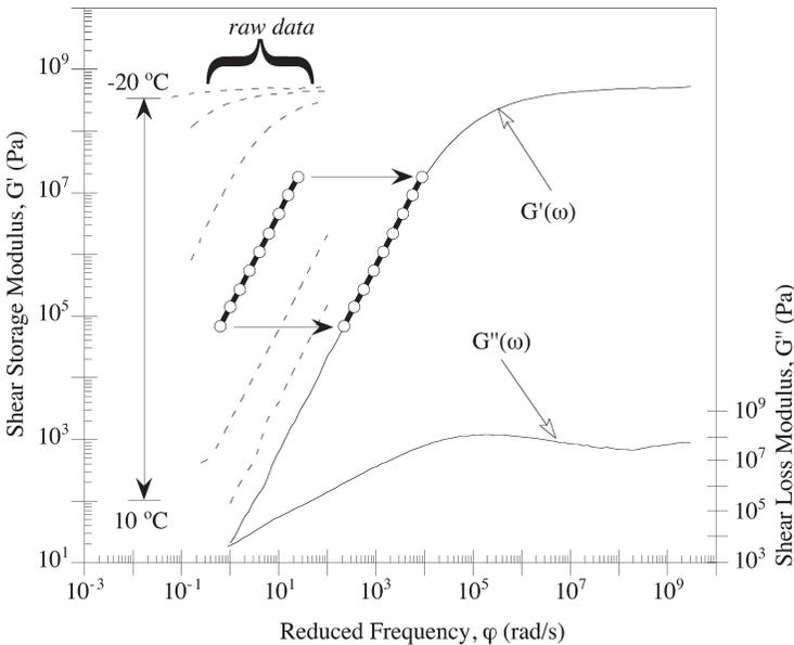
**Figure 3.** Dynamic shear moduli master curve construction,  $\alpha = 0.22$ ,  $T_{ref} = 10^\circ\text{C}$ .
