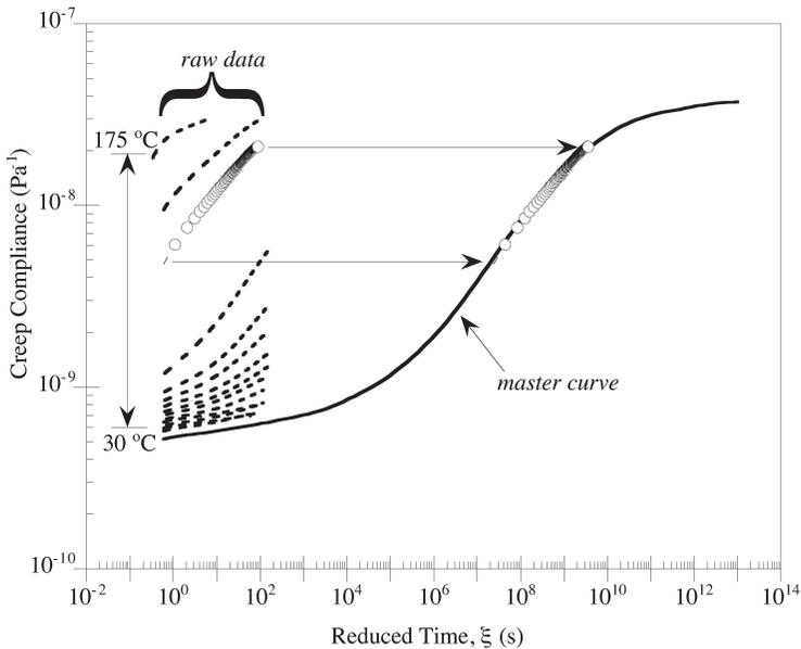
**Figure 4.** Creep compliance master curve construction,  $\alpha = 1.0$ ,  $T_{\text{ref}} = 30^{\circ}\text{C}$ .
