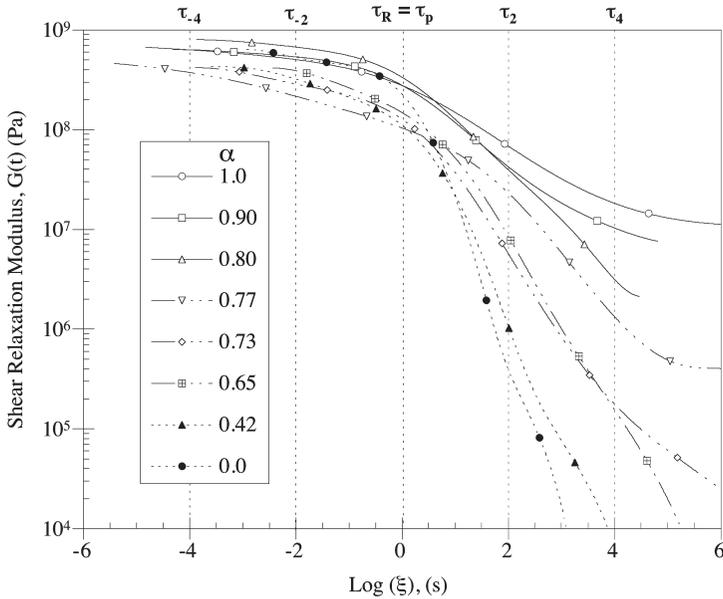
**Figure 12.** Shear relaxation modulus at each cure state after shifting to the reference time,  $\tau_p$ .
