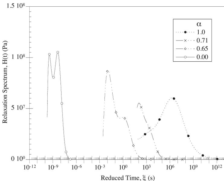
Figure 10. Relaxation spectrum of EPON 862/W over the entire range of cure,  $T_{ref} = 30^\circ\text{C}$ .
