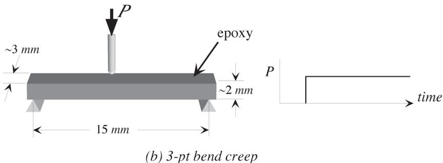
**Figure 2 (continued).** Experimental setups used in this study: (a) oscillatory shear between parallel plates and (b) creep under three-point bending.
