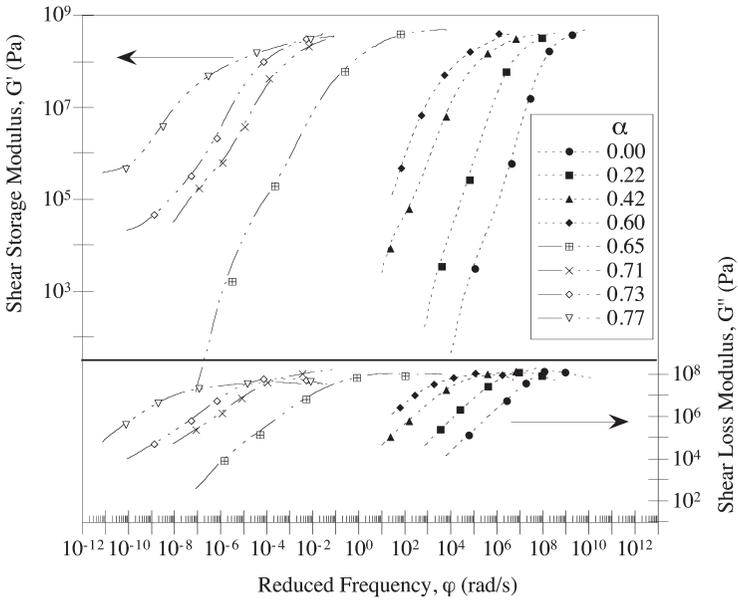
**Figure 5.** Dynamic moduli master curves from oscillatory shear experiments,  $T_{ref} = 30^{\circ}C$ .
