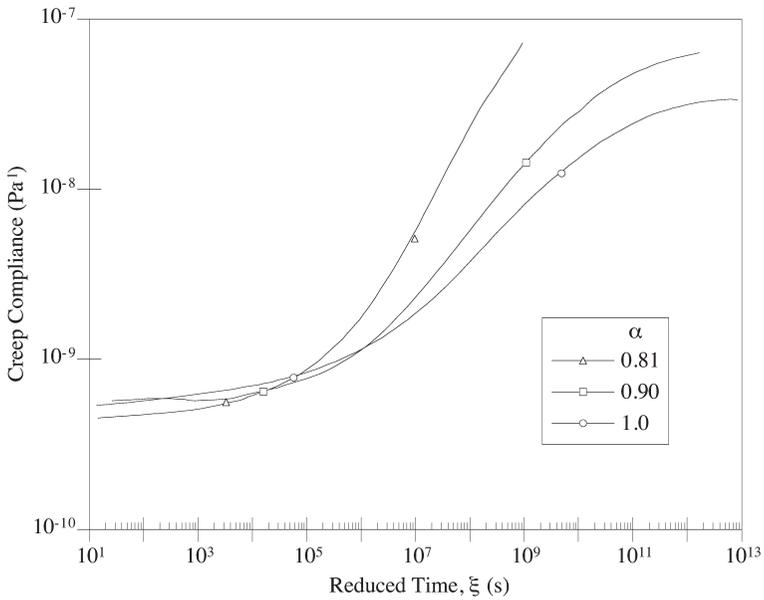
**Figure 6.** Creep compliance master curves determined by creep testing of 3-point bend specimens,  $T_{ref} = 30^{\circ}C$ .
