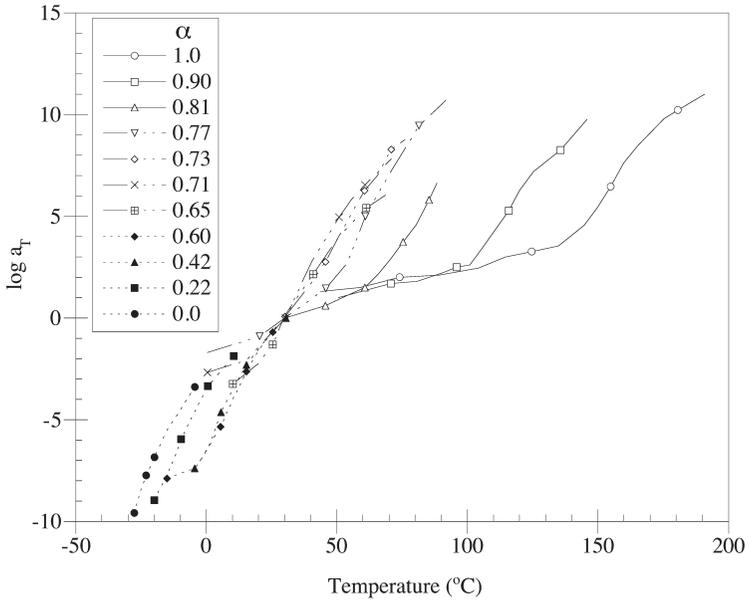
**Figure 7.** Shift factors used in constructing master curves,  $T_{ref} = 30^{\circ}C$ .
