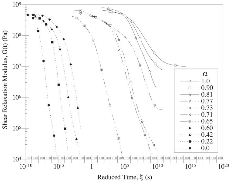
**Figure 9.** Shear relaxation modulus of EPON 862/W over the entire range of cure,  $T_{\text{ref}} = 30^\circ\text{C}$ .
