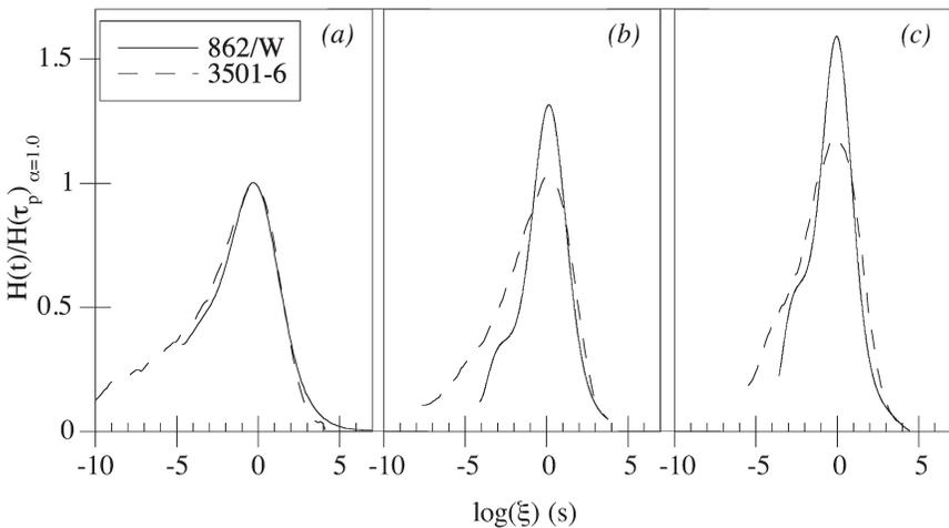
**Figure 15.** Relaxation spectra normalized by  $H(\tau_p)_{\alpha=1.0}$  for EPON 862/W and Hercules 3501-6 [10] at various cure states: (a)  $\alpha = 1.0$ , (b)  $\alpha \approx 0.90$ , (c)  $\alpha \approx 0.80$ .
