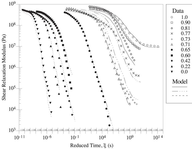
**Figure 14.** Correlation between the experimental data and the cure dependent model proposed in Equation (15).
