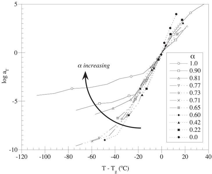
**Figure 8.** Shift factors used in constructing master curves,  $T_{ref} = T_g$ .
