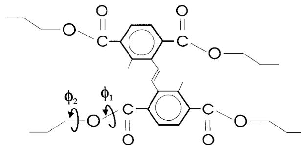
Fig. 10. Schematic of two neighboring PET chains that have been coupled via a BCB-BCB crosslinking reaction.  $\phi_1$  and  $\phi_2$  are torsional angles about which rotation may be activated during the  $\beta$  relaxation process.
