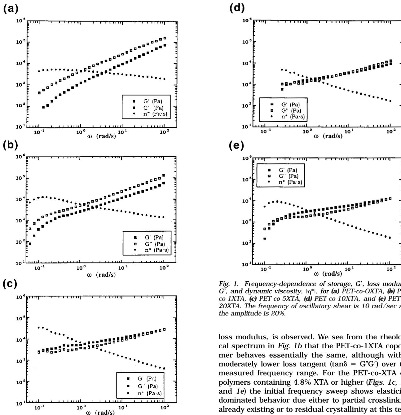
Fig. 1. Frequency-dependence of storage,  $G'$ , loss modulus,  $G''$ , and dynamic viscosity,  $|\eta^*|$ , for (a) PET-co-OXTA, (b) PET-co-1XTA, (c) PET-co-5XTA, (d) PET-co-10XTA, and (e) PET-co-20XTA. The frequency of oscillatory shear is 10 rad/sec and the amplitude is 20%.
