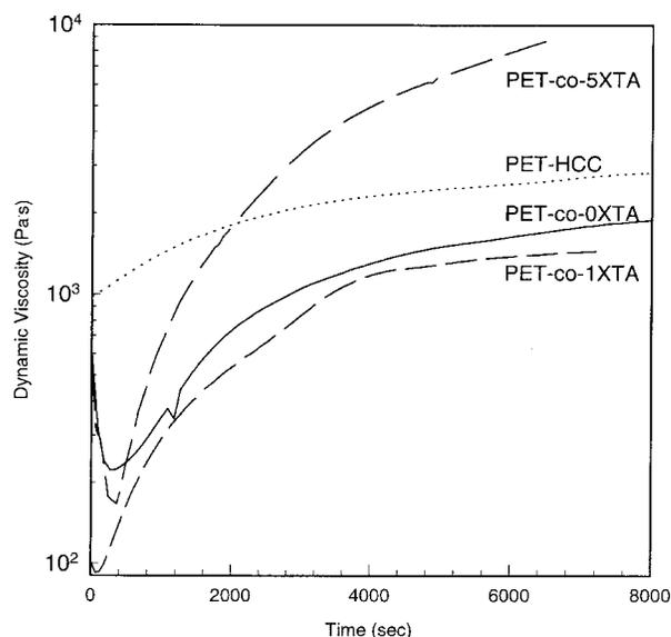
Fig. 7. Comparison of the dynamic viscosity evolution at  $275^{\circ}\text{C}$  for all of the PET-co-XTA copolymers, as well as a commercial grade PET. The oscillation frequency is 10 rad/sec and the strain amplitude varies from 2% (5XTA) to 20% (1XTA).
