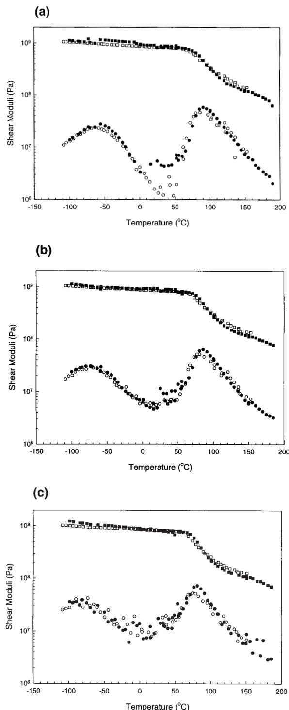
Fig. 8. Temperature dependence of the shear storage ( $\square$ ) and shear loss ( $\circ$ ) moduli of PET-co-5XTA molded at 275°C for 2 minutes (filled symbols) and for 120 minutes (open symbols). The oscillation frequency is (a) 100 (b) 10, and (c) 1 rad/sec.
