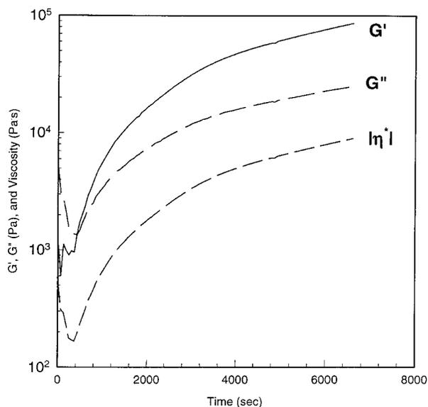
Fig. 6. Time dependence of the rheological material functions of PET-co-5XTA at  $T = 275^{\circ}\text{C}$ . The oscillation frequency is 10 rad/sec and the strain amplitude is 2%.
