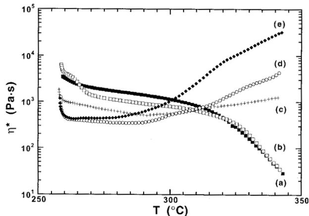
Fig. 3. Temperature-dependence of the dynamic viscosity,  $|\eta^*|$ , for (a) PET-co-OXTA, (b) PET-co-1XTA, (c) PET-co-5XTA, (d) PET-co-10XTA, and (e) PET-co-20XTA. The oscillation frequency is 10 rad/sec, the strain amplitude is 20%, and the heating rate is  $5^\circ\text{C}/\text{min}$ .
