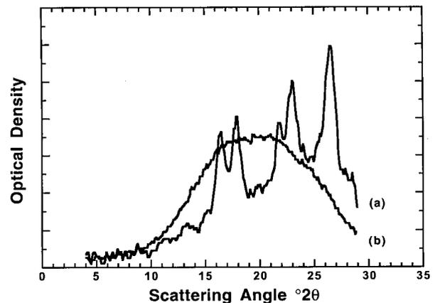
Fig. 13. Line profiles of wide-angle X-ray scattering (WAXS) patterns for PET-co-5XTA at room temperature (a) before crosslinking, and (b) after crosslinking at 275°C for 120 minutes.
