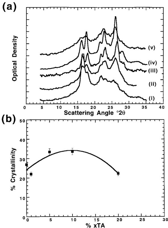
Fig. 12. (a) Line profiles of wide-angle X-ray scattering (WAXS) data shown in Fig. 11: (i) PET-co-OXTA, (ii) PET-co-1XTA, (iii) PET-co-5XTA, (iv) PET-co-10XTA, and (v) PET-co-20XTA. (b) Percentage crystallinity versus mole-percentage XTA comonomer.
