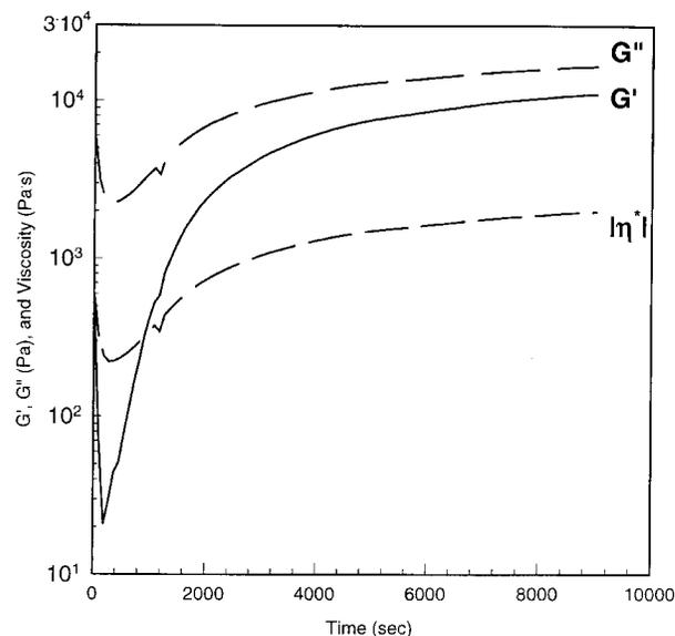
Fig. 4. Time dependence of rheological material functions of PET-co-OXTA at  $T = 275^\circ\text{C}$ . The oscillation frequency is 10 rad/sec and the strain amplitude, determined to be within linear limits, is 10%.
