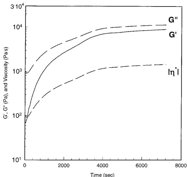
Fig. 5. Time dependence of the rheological material functions of PET-co-1XTA at  $T = 275^{\circ}\text{C}$ . The oscillation frequency is 10 rad/sec and the strain amplitude, determined to be within linear limits, is 20%.
