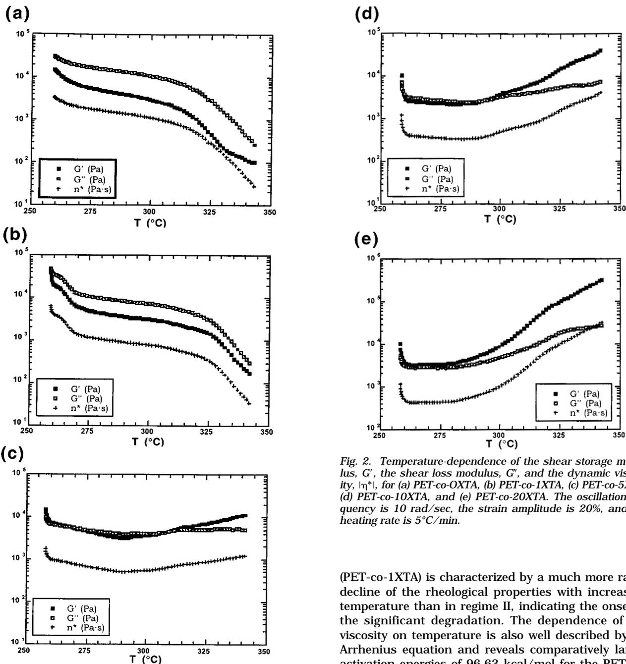
Fig. 2. Temperature-dependence of the shear storage modulus,  $G'$ , the shear loss modulus,  $G''$ , and the dynamic viscosity,  $\ln^*$ , for (a) PET-co-0XTA, (b) PET-co-1XTA, (c) PET-co-5XTA, (d) PET-co-10XTA, and (e) PET-co-20XTA. The oscillation frequency is 10 rad/sec, the strain amplitude is 20%, and the heating rate is 5°C/min.
