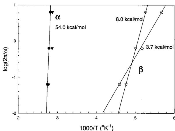
Fig. 9. Arrhenius plots yielding the activation energies of the  $\alpha$  (filled) and  $\beta$  (open) mechanical relaxations for the 5XTA sample annealed for 2 minutes (○) and for 120 minutes (▽) at 275°C.
