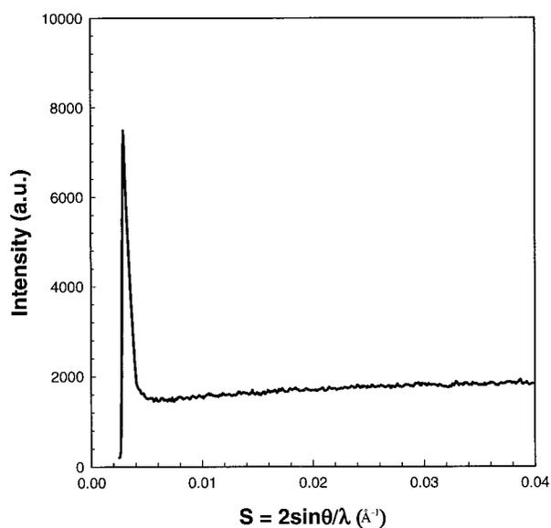
Figure 13. Small angle X-ray scattering (SAXS) of 8 mol % CyPOSS (**3a**) at  $T = 240^{\circ}\text{C}$ . See text for details.
