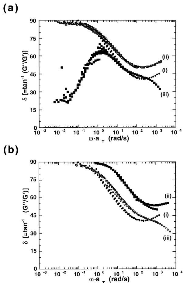
**Figure 10.** Loss angle,  $\delta$ , as a function of frequency,  $\omega$ , at 180°C. (a) Copolymers with (i) 0, (ii) 4, and (iii) 8 mol % CyPOSS content. (b) Copolymers with (i) 0, (ii) 4, and (iii) 8 mol % CpPOSS content.
