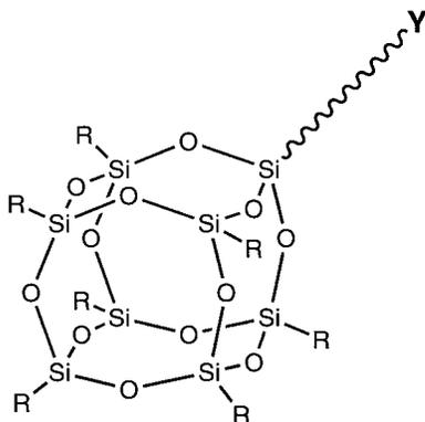
**Figure 1.** A representative POSS macromer with seven solubilizing R groups and a single Y group for incorporation into a polymer. Such a POSS macromer is used to make a hybrid polymer with a pendant architecture.
