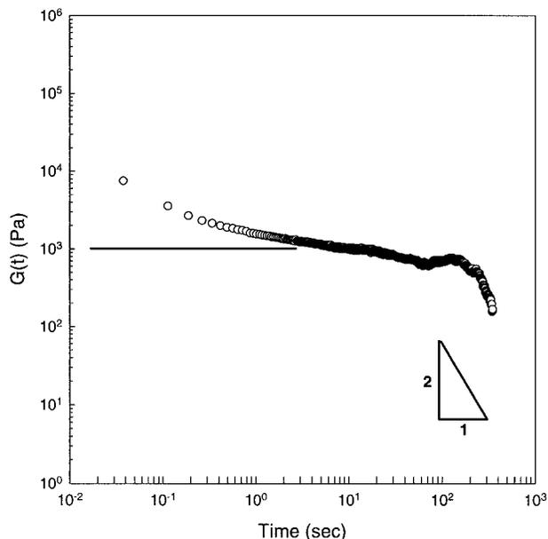
**Figure 8.** Shear stress relaxation following step shear strain for the 8 mol % CyPOSS copolymer (sample **3a**). The strain amplitude,  $\gamma_o$ , is 0.2 and  $T = 240^\circ\text{C}$ .
