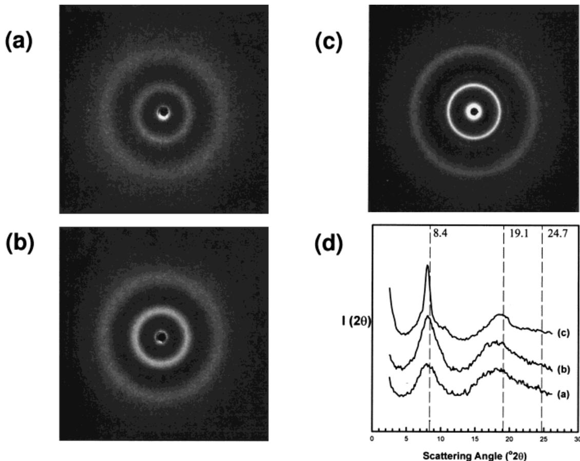
**Figure 4.** Wide-angle X-ray scattering patterns of as-polymerized CpPOSS copolymers of (a) 4 (**4b**), (b) 8 (**3b**), and (c) 17 (**2b**) mol % POSS content. (d) Optical density as a function of scattering angle  $2\theta$  of the patterns shown in (a)–(c) Cu target and graphite monochromator were used.
