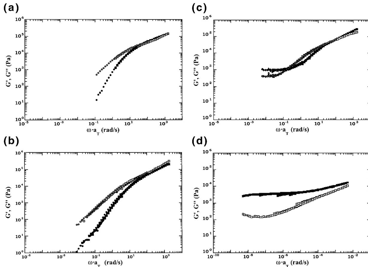
**Figure 7.** Dynamic moduli  $G'(\omega)$  (filled symbols),  $G''(\omega)$  (open symbols) master curves for (a) polymethylstyrene (**5**), and (b) 4 (**4a**); (c) 8 (**3a**); and (d) 17 (**2a**) mol % CyPOSS copolymers at a reference temperature of 180°C.
