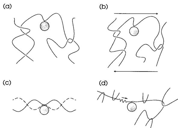
Figure 14. Schematic illustration of potential inertial effects resulting from POSS-incorporation along a polymer backbone. (a) The unstressed state, (b) following an abrupt shearing deformation, (c) Rouse mode modification, and (d) modification of reptation.
