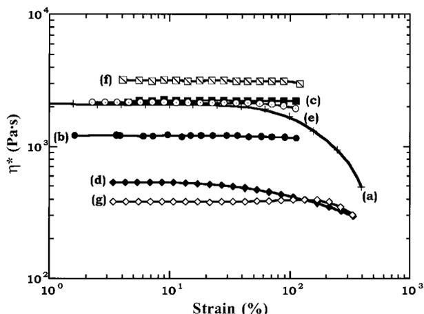
**Figure 6.** Dynamic viscosity  $|\eta^*|$  as a function of strain,  $\gamma$ , for (a) polystyrene (**5**) and (b) 4 (**4b**); (c) 8 (**3b**); (d) 15 (**2b**) mol % CpPOSS copolymers, and (e) 4 (**4a**); (f) 8 (**3a**); and (g) 17 (**2a**) mol % CyPOSS copolymers. Data measured at 10 rad/s and 180°C (a)–(e), 200°C (f) and 300°C (g).
