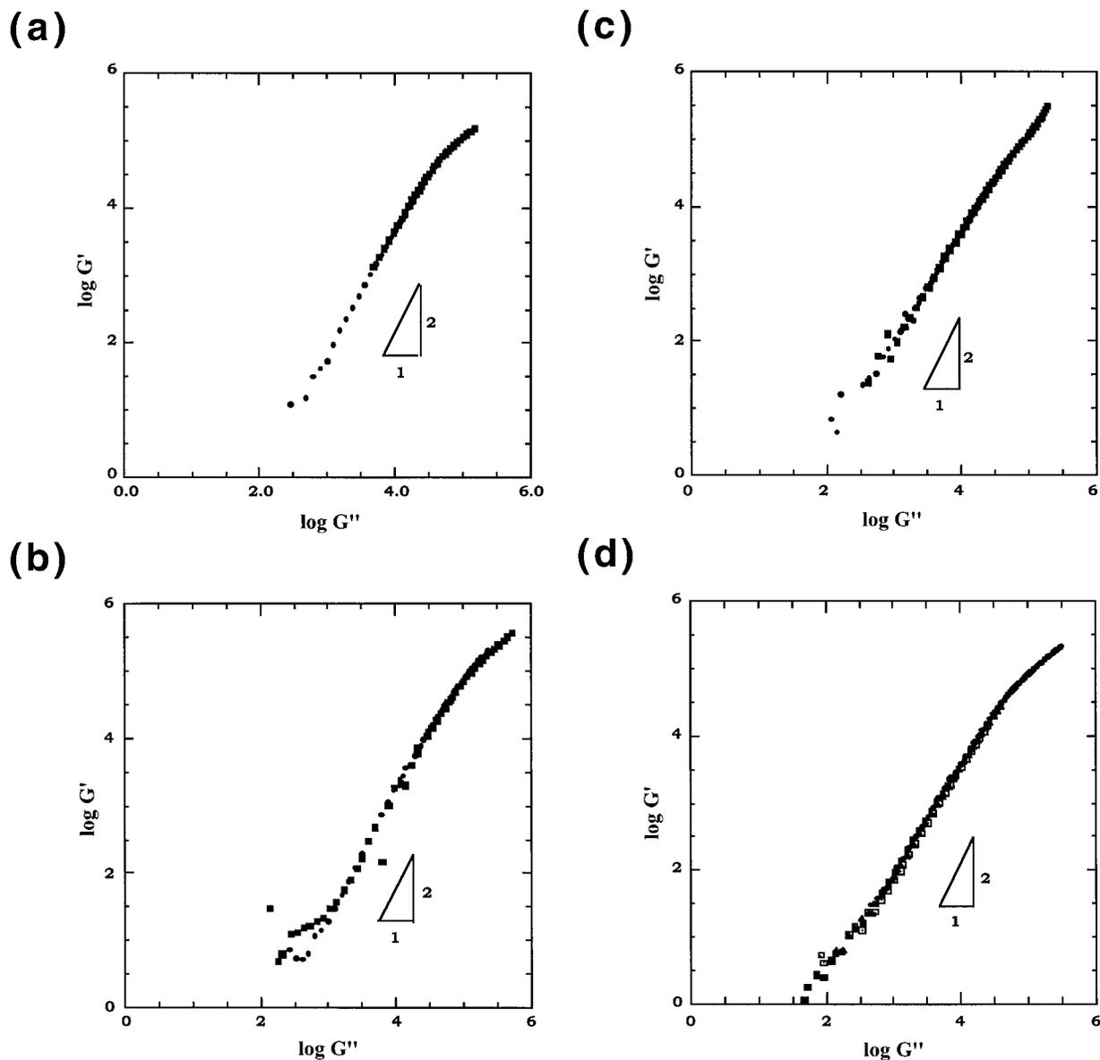
**Figure 12.**  $\log G'(\omega)$  as a function of  $\log G''(\omega)$  for (a) polystyrene (**5**), and (b) 4 (**2b**), and (c) 8 (**3b**) mol % CpPOSS copolymers, and (d) 4 (**2a**) and (e) 8 (**3a**) mol % CyPOSS copolymers. The slopes corresponding to the linear (terminal) region in each plot are (a) 1.76; (b) 1.89; (c) 1.57; and (d) 1.50.
