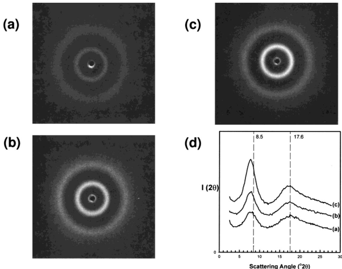
**Figure 5.** Wide-angle X-ray scattering patterns of as-polymerized CyPOSS copolymers of (a) 4 (**4a**), (b) 8 (**3a**), and (c) 15 (**2a**) mol % POSS content. (d) Optical density as a function of scattering angle  $2\theta$  of the patterns shown in (a)–(c). Copper target and graphite monochromator were used.
