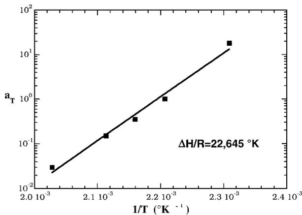
**Figure 11.** Arrhenius plot of viscosity shift factor,  $a_T$  ( $=\eta(T)/\eta(T_{\text{ref}})$ ), for 4 mol % CyPOSS (**2a**).
