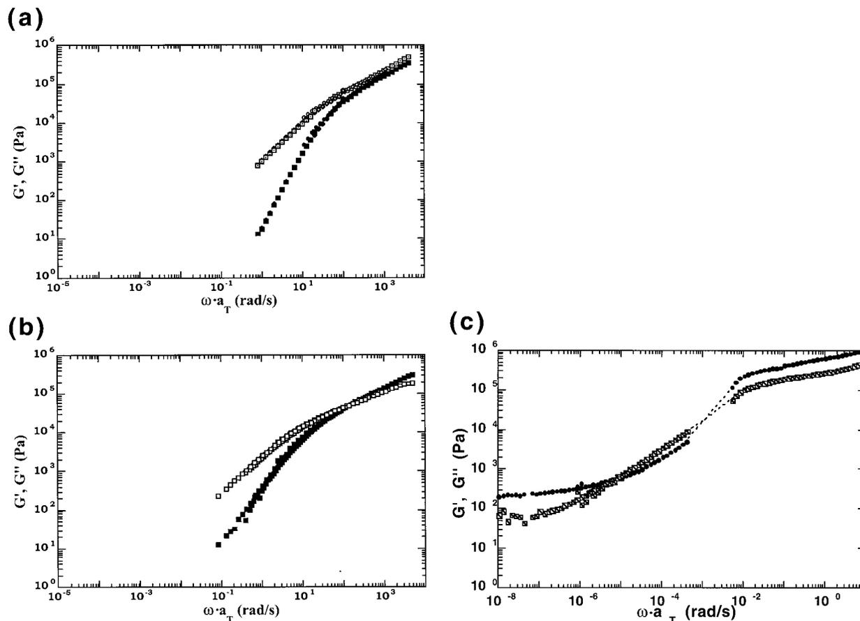
**Figure 9.** Dynamic moduli  $G'(\omega)$  (filled symbols),  $G''(\omega)$  (open symbols) master curves for (a) 4 (**4b**); (b) 8 (**3b**); and (c) 16 (**2b**) mol % CpPOSS copolymers at a reference temperature of 180°C.
