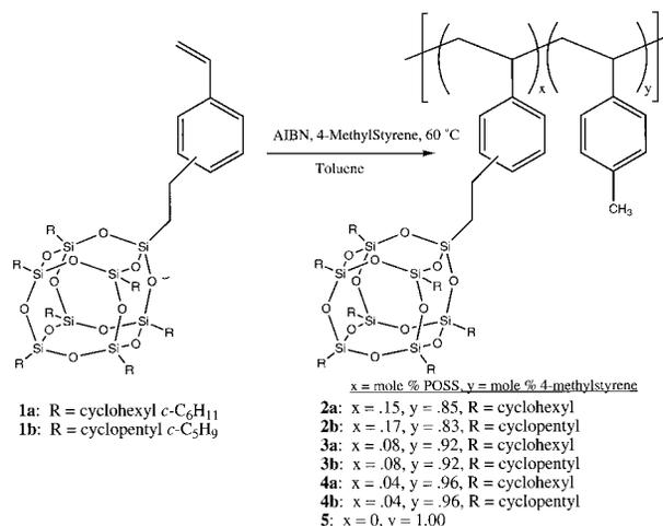
**Figure 2.** POSS styryl macromer copolymerization.
